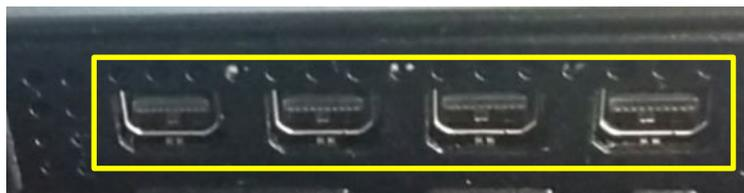
Use a **Mini Display Port** to Display Port adapter cable to connect the monitor to the PC. Ensure the Adaptor cable supports 4K@60Hz.
